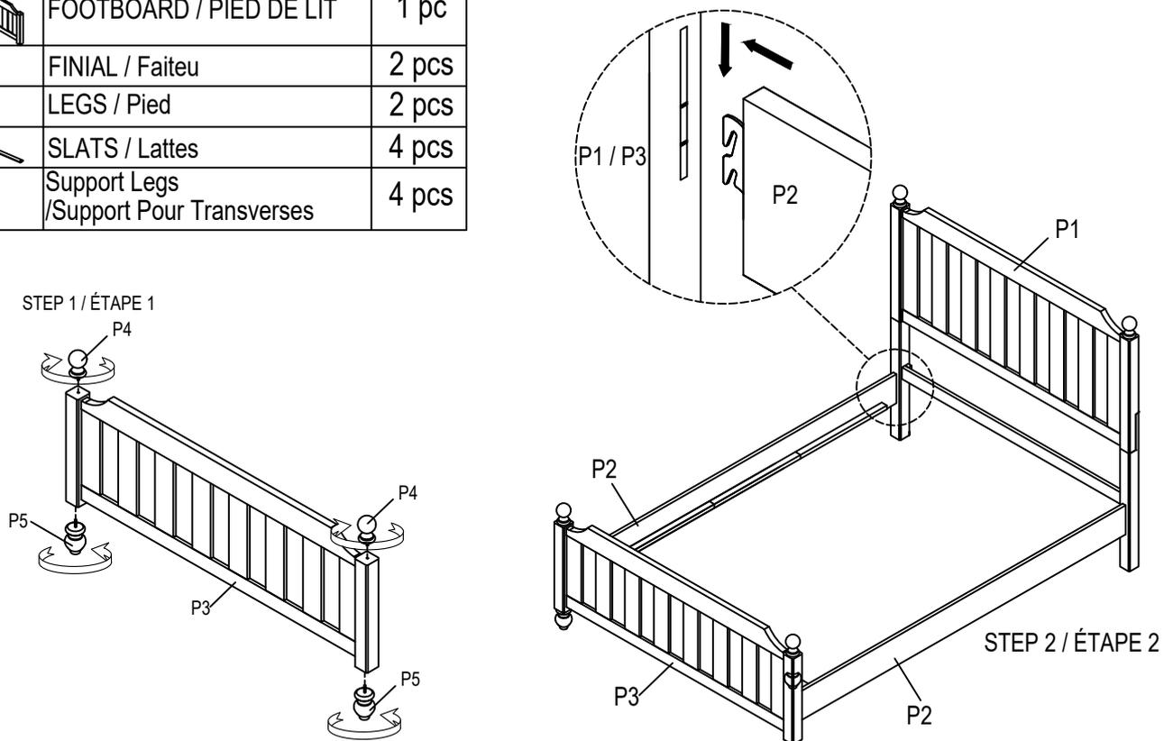
DONOT TIGHTEN BOLTS UNTIL COMPLETELY ASSEMBLED
