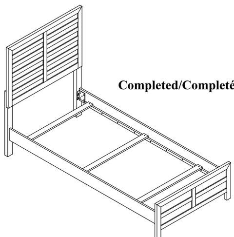
**\*\*DO NOT TIGHTEN BOLTS UNTIL COMPLETELY ASSEMBLED
