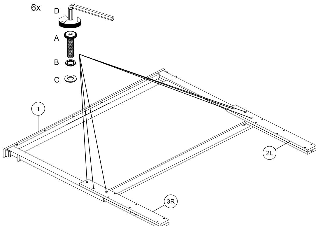
DO NOT TIGHTEN BOLTS UNTIL COMPLETELY ASSEMBLED.
