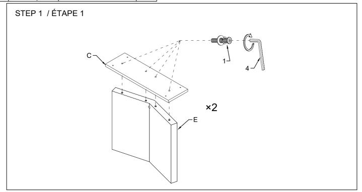
DO NOT TIGHTEN BOLTS UNTIL COMPLETELY ASSEMBLED.
