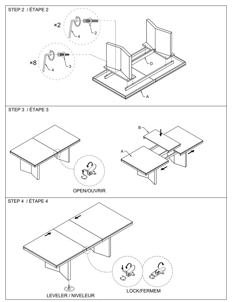
DO NOT TIGHTEN BOLTS UNTIL COMPLETELY ASSEMBLED.
