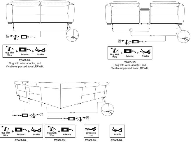
Plug with wire, adaptor, and Y-cable unpacked from LRPWH.
