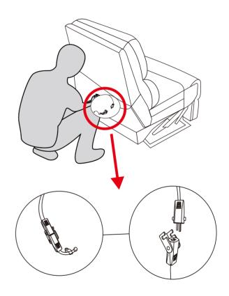
Please check and connect the power port of seat motor and headrest motor, make sure secure the protector.
