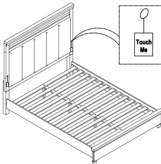
DO NOT TIGHTEN BOLTS UNTIL COMPLETELY ASSEMBLED.
