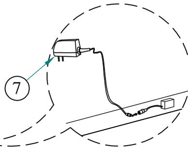
Ensure adapter socket connect to behind mirror socket /
