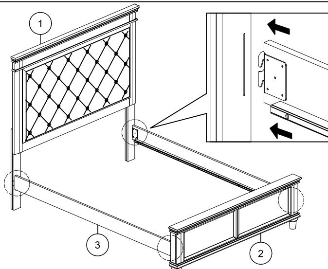
**DO NOT TIGHTEN BOLTS UNTIL COMPLETELY ASSEMBLED.
