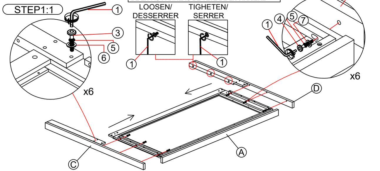
**STEP 1:1** Attach the Headboard Leg (C) and Headboard Leg (D) to Headboard (A) as shown using JCBC Bolt (3), Spring Washer (5), Flat Washer (6) and fasten with Allen Wrench (1).
