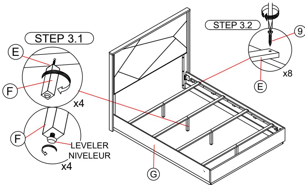
**STEP 3:1** Fix the Bed Slats Support (F) to Bed Slats (E) as Shown, Loosen or Tighten the Adjuster as necessary to level the Bed
