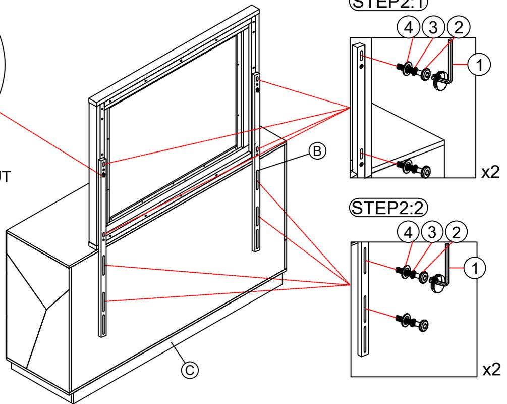
**STEP 2:1** Attach Mirror Support Rail (B) to Mirror (A) as shown using JCBC Bolt (2), Spring Washer (3), Flat Washer (4) and fasten with Allen Wrench (1)
