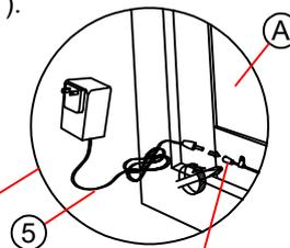
Loosen the screw to connect
