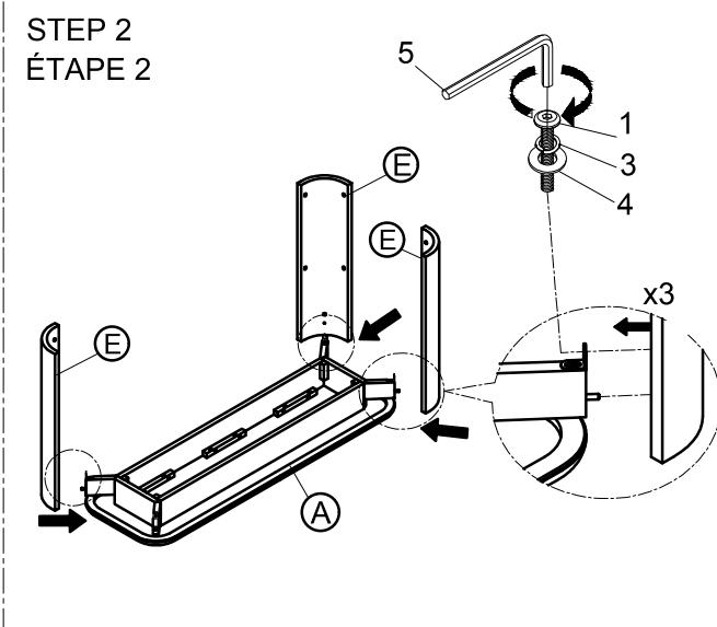
Do not tighten bolts until completely assembled
