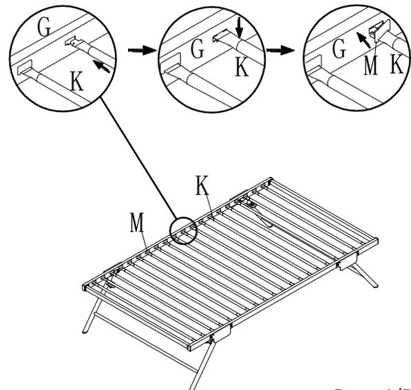
Note: Please do not tighten all bolts until the bed is assembled completely.
