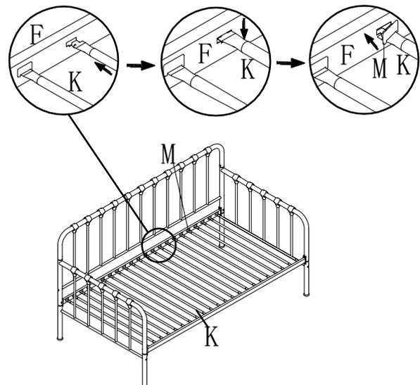
Note: Please do not tighten all bolts until the bed is assembled completely.
