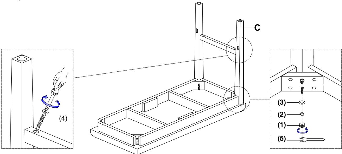
DO NOT TIGHTEN BOLTS UNTIL COMPLETELY ASSEMBLED.
