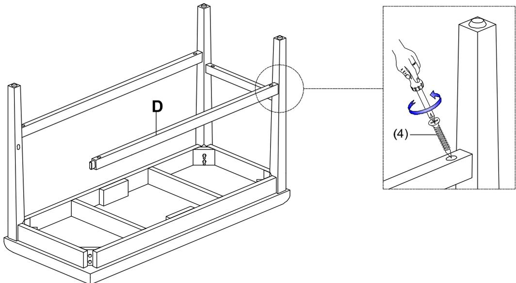
DO NOT TIGHTEN BOLTS UNTIL COMPLETELY ASSEMBLED.
