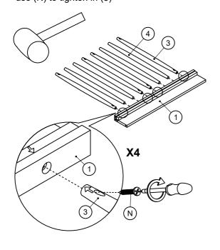
used plastic hammer insert 2 into (3) and (4) and use (N) to tighten in (3)
