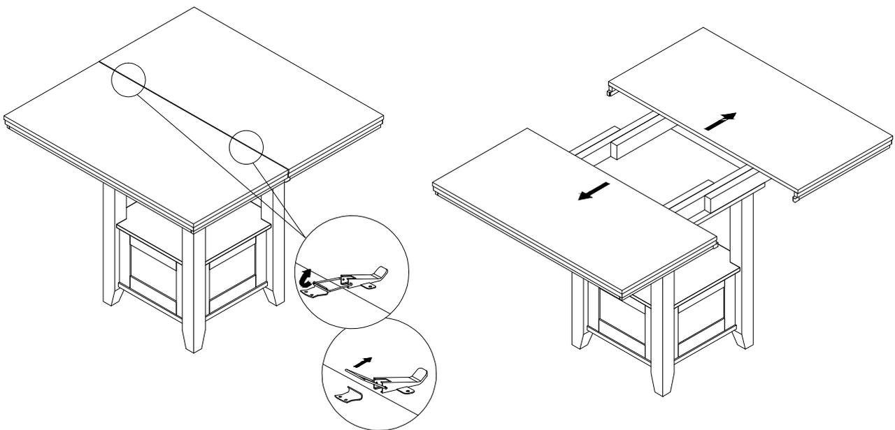
**DO NOT TIGHTEN BOLTS UNTIL COMPLETELY ASSEMBLED.**
