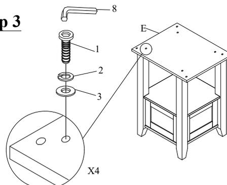
**DO NOT TIGHTEN BOLTS UNTIL COMPLETELY ASSEMBLED.
