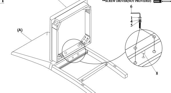
DO NOT TIGHTEN BOLTS UNTIL COMPLETELY ASSEMBLED.
