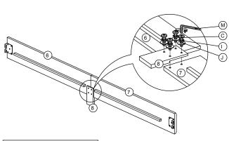
Do not fully tighten screws until assembly is complete and the bed is level.
