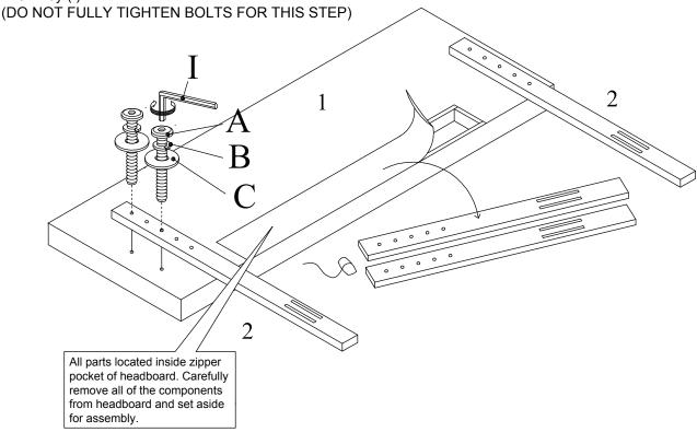
Attached Bed Rails (not included) to left and right Headboard Legs (2) using 2 Allen bolts (D) and 2 Flat Washer (F) from the back and 2 Flat Washer (F), 2 Lock Washer (E) and 2 Hex Nuts (G) from the front. Tighten all bolts with Allen Key (H) provided.
