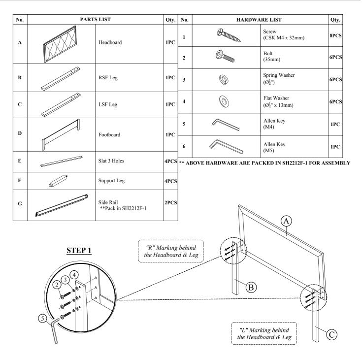
DO NOT TIGHTEN BOLTS UNTIL COMPLETELY ASSEMBLED.
