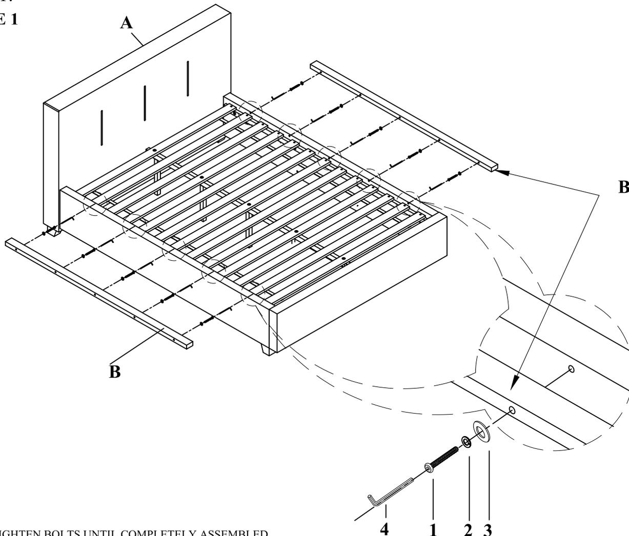
\* DO NOT TIGHTEN BOLTS UNTIL COMPLETELY ASSEMBLED
